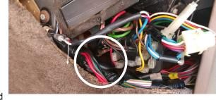
Route the Green "Mod Switch" wire along the underside of the dashboard
