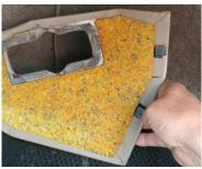
Remove the Left/ & Right hand side under -dash closing panel by removing 4 retaining screws.
